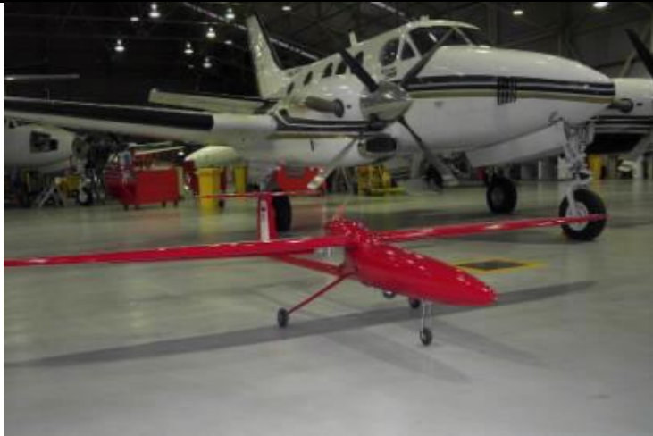
Flamingo ready for Outback Challenge 2007. Note camera blister under the fuselage and the pitot head in the nose.
