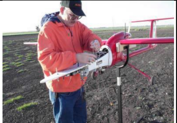
Dave Jones (AUAV) working on the Flamingo prior to the Outback Challenge 2007. Note the ease of access to the avionics using the pannier style nose configuration and a sensible stand.
