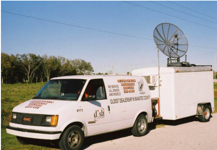
AUAV Ground Station Van. Note the video dish mounted GCS trailer. A very nicely set-up GCS
