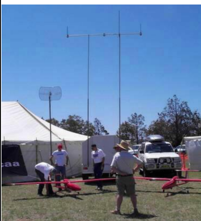
Antenna array used in the Outback Challenge 2007. This array included antennas for the video, control and duplex data transmitters.
