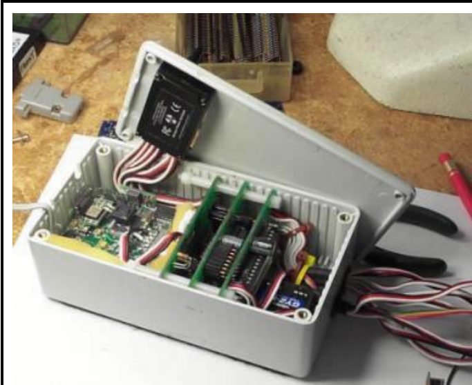
Ezi-Nav Autopilot showing interior modified by Silvertone to include IMU and a 2.4GHz RX
